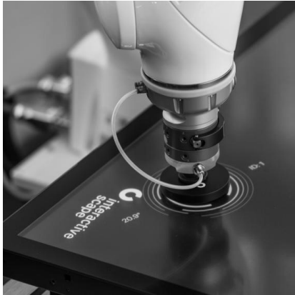
Fig. 4. The Multitouch Displays Scape® Tangible, which is the display used in the robotic training station [28].
